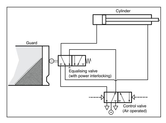
Figure 10 Use of an equalising valve - power locking (guard open)
