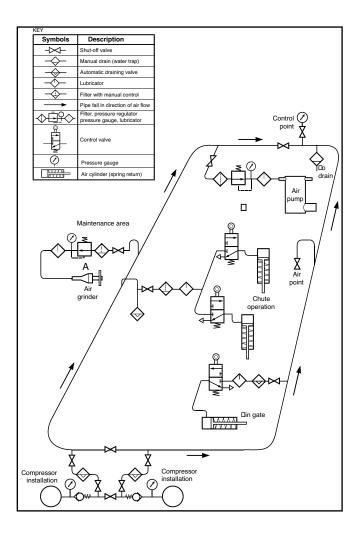
Figure 3 Ring main system - typical layout
