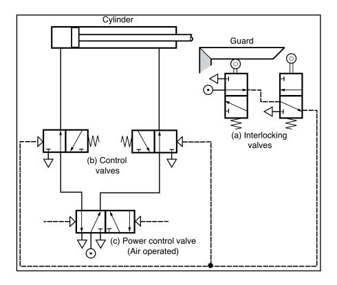
Figure 7 Single control system interlocking with piston arrest and hold (guard closed)
