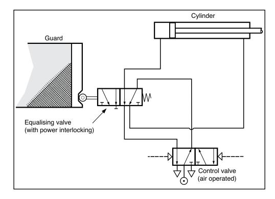
Figure 11 Use of an equalising valve - power locking (guard closed)
