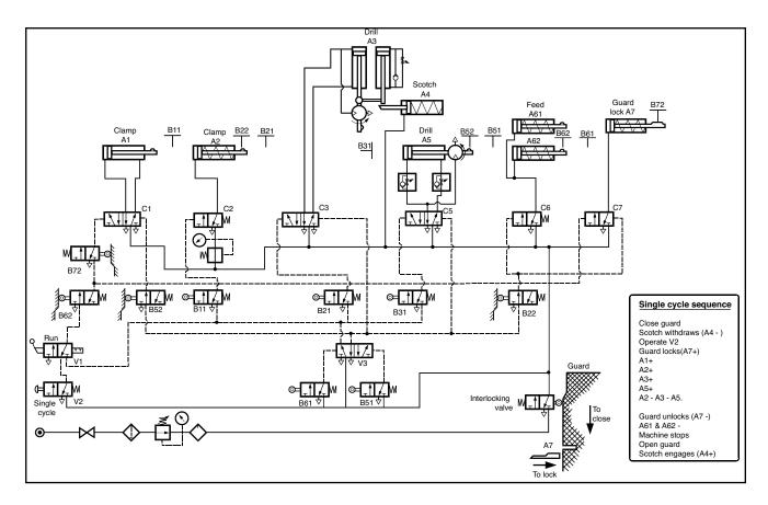
Figure 19 Guard operated power interlocking with scotch to prevent drill falling under gravity. Also fitted with guard lock to prevent inadvertent opening
