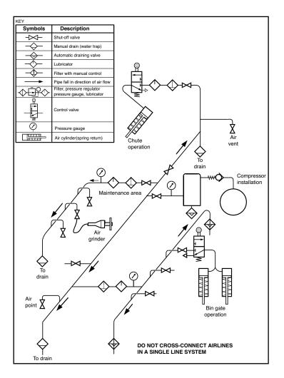
Figure 2 Single line system - typical layout
