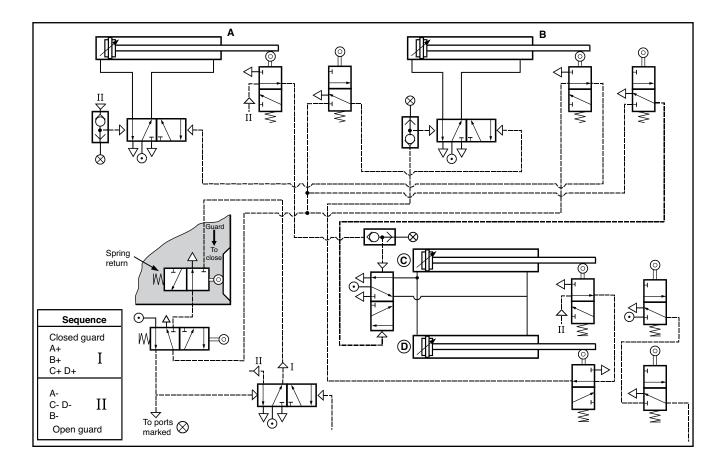
Figure 14 Control system interlocking from complex sequence
