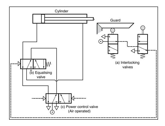
Figure 9 Use of an equalising valve - control interlocking (guard closed)
