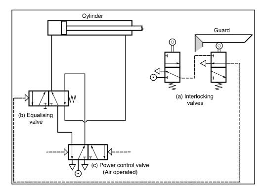
Figure 8 Use of an equalising valve - control interlocking (guard open)
