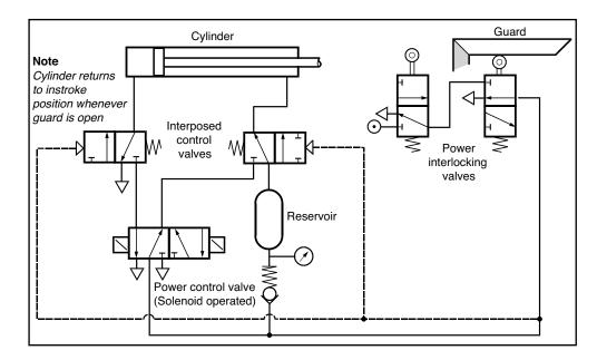
Figure 12 Use of a reservoir - power interlocking (guard open)
